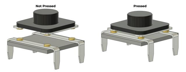
When the button is not pressed there is not an electrical connection between the pins on the left and the pins on the right side of the button. When the button is pressed, all the pins are connected electrically.
