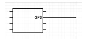
When nothing is connected to the Pin's input, we call that "floating". It's not clear what the microcontroller should detect, so it often flickers between LOW and HIGH. These flickering readings can really mess with your program – more on that in a bit!
