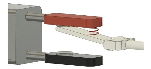
But when you connect the input to ground by pressing your pushbutton, the connection pulls harder to Ground (0 Volts), overcoming the internal pull-up:
