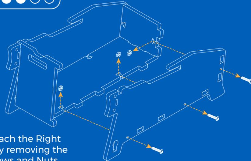
Detach the Right side by removing the Screws and Nuts
